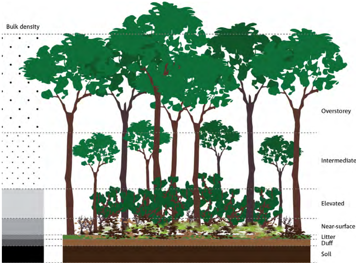
Figure 12 Schematic diagram illustrating the broad categories of forest fuel strata present in a forest. (Source: Gould et al. 2011)
